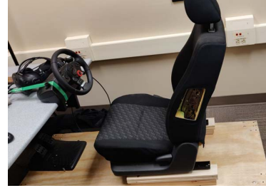
Figure 2: Car seat, steering wheel and pedal setup
