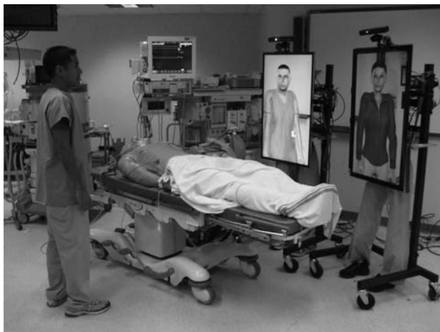
Figure 2. High-physicality condition. The pair of ANDI units display the characters at life-size where they should stand, and use a combination of a see-through display and physical legs to create the sense that the ECAs share the physical space.
