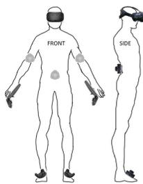
Figure 3: HTC Vive HMD, controller and tracker placement on participant. Grayed out trackers were placed on the lower back and just above the elbows on the back of the arm of the participant.
